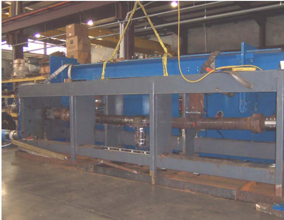
Figure 13 – Photograph of pressure-tension-bending load frame test set-up
