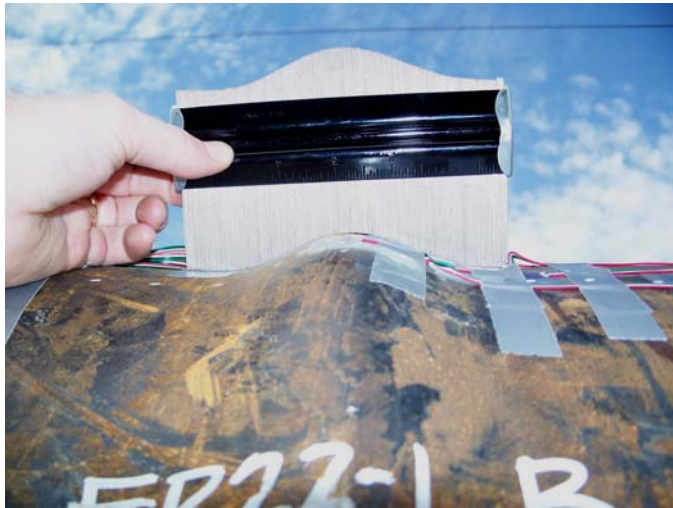
Figure 2 – Measurement made using steel profile comb
