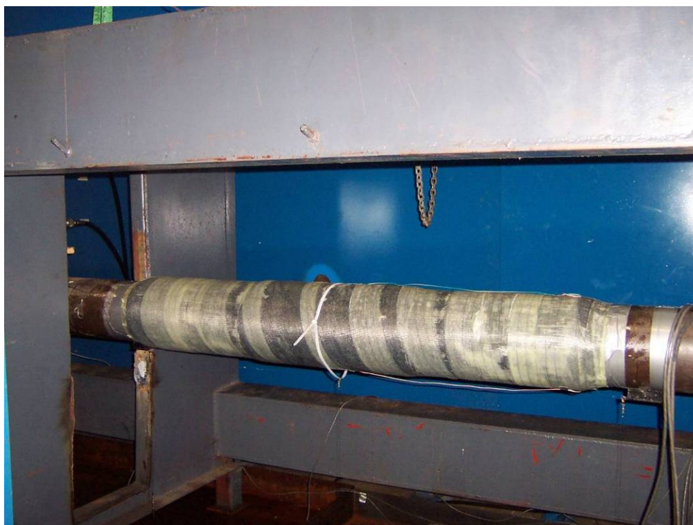
Figure 12 – Photo showing Product C prior to bend testing
