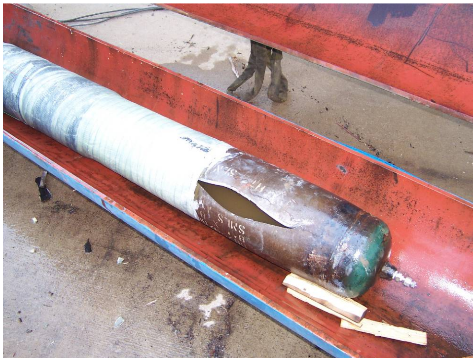
Figure 8 – Failure in burst sample using Product C
