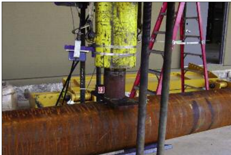
Figure 1. Dent installation rig to install dents.
