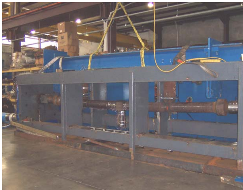
Figure 2 – Images of pressure-tension-bending load frame test set-up
