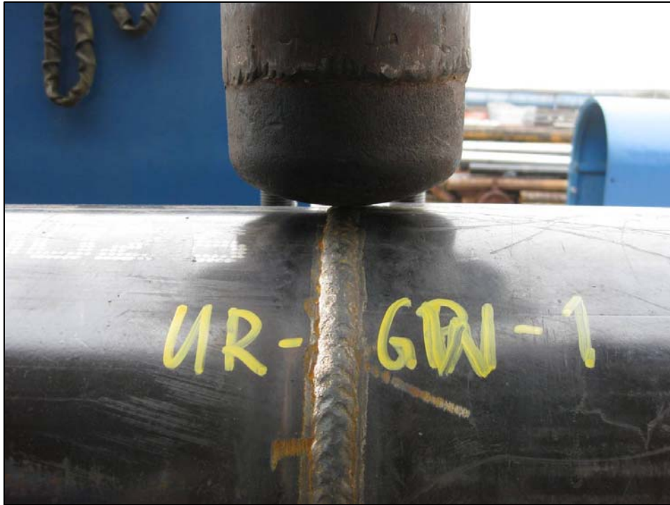
Figure 3 – Close-up view on indenter on girth weld
