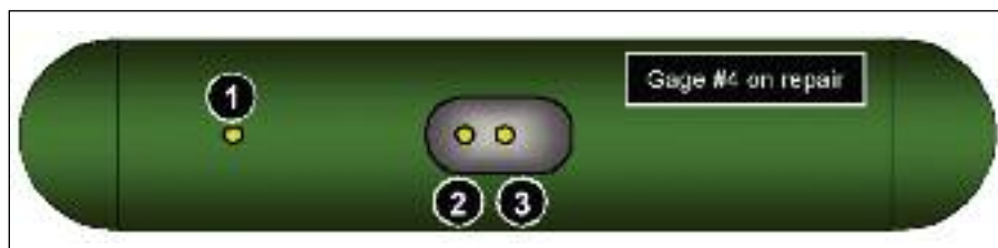
Figure 2. Diagram of strain gage locations.
